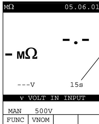
ATTENTION: the test can't be executed. Check that the circuit is not energized.
