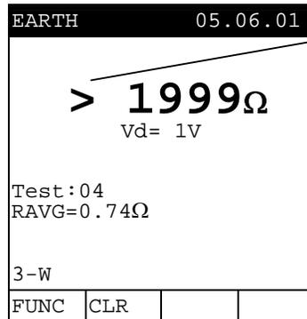
Message ">1999" means that the resistance value is higher than the maximum measurable.
