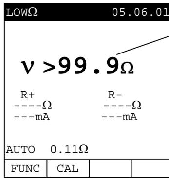
Message **>99.9Ω:** means that the instrument detected a resistance higher than 5Ω therefore it will proceed with Reset procedure.
