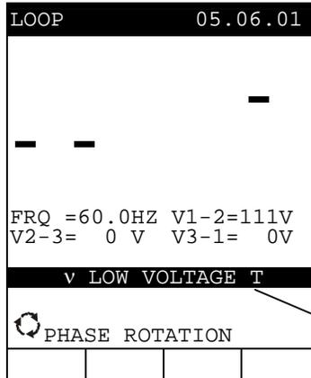
Phase "T2 Voltage is lower than 100V
