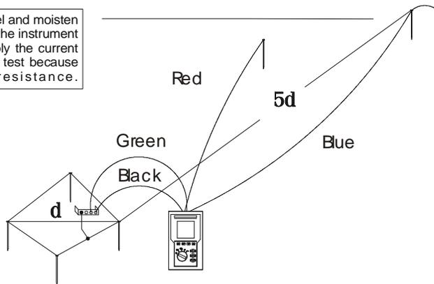
**Ground resistance measurement for small Ground plant**
