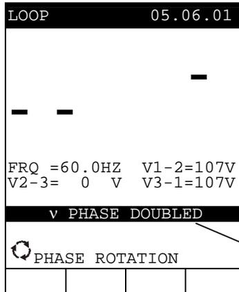
Two phases are connected together.
