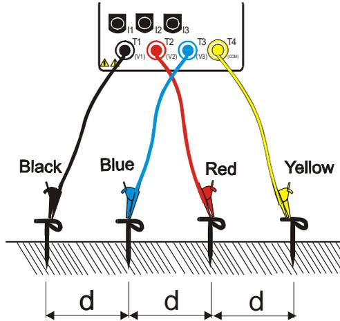
Instrument connection for Earth resistivity measurement
