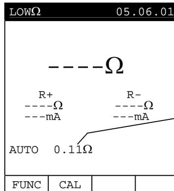
A numerical value in this field means that the instrument has been calibrated; this value **remains on the display for any further measurement** even though the unit is switched off and on again.
