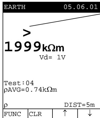
Message ">1999" means that the resistivity value is higher than the maximum measurable.
