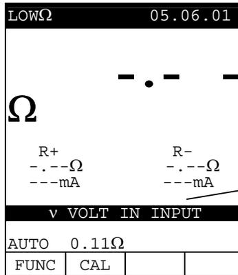
ATTENTION: the test was not performed because of voltage at the terminal ends.
